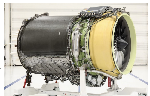
Two of the latest contenders for the B-52 engine program are the Rolls-Royce F130 (top) and the General Electric Passport (above). Both will fit the current nacelle configuration with minimal modifications.
