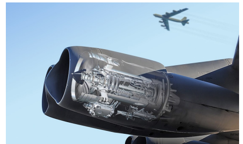
Numerous engines have been proposed for the B-52 over the years such as the Pratt & Whitney J75, Rolls-Royce RB211-535 and the CFM International CFM56 with different designations having been applied to the re-engined aircraft including B-52I, B-52R & B-52RE. (Photo/Illustration by Erik Simonsen)
