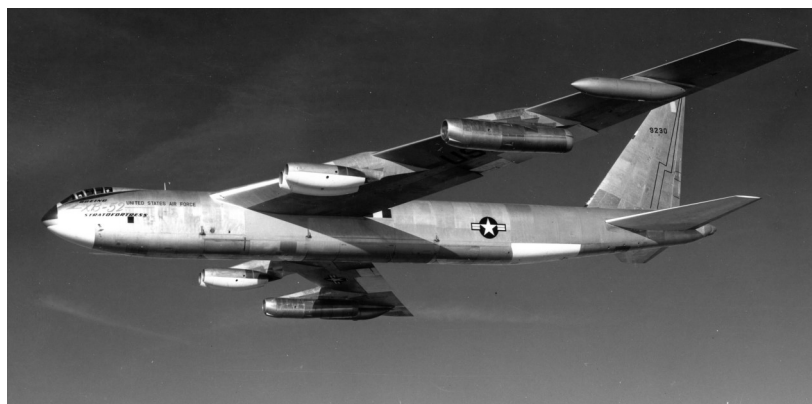
The Boeing prototype XB-52 was utilized for a series of tests utilizing an afterburner-equipped J75 engine on the outboard wing pylons. (Boeing)
